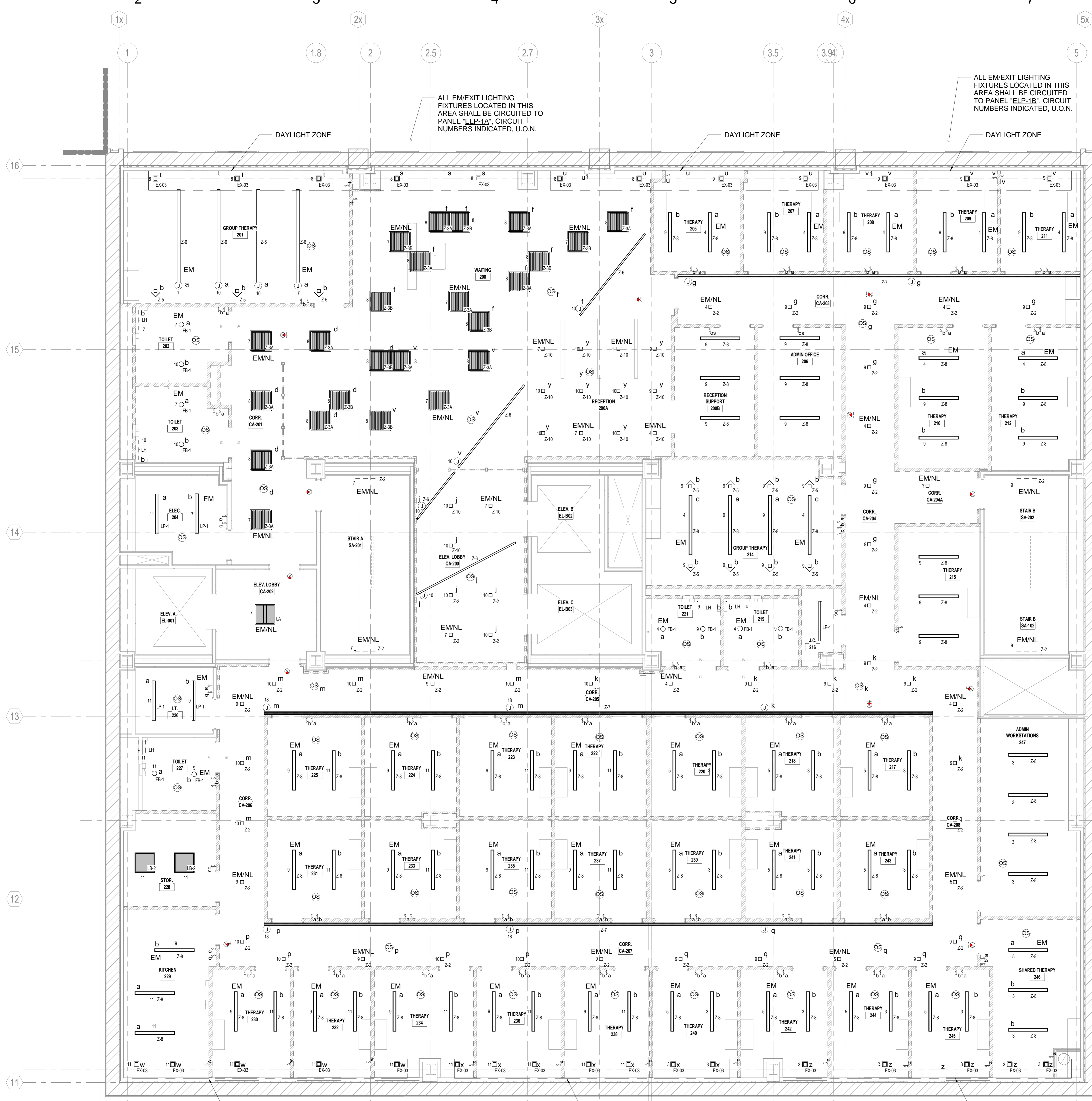
1 SECOND FLOOR LIGHTING PLAN 1/4" = 1'-0"
