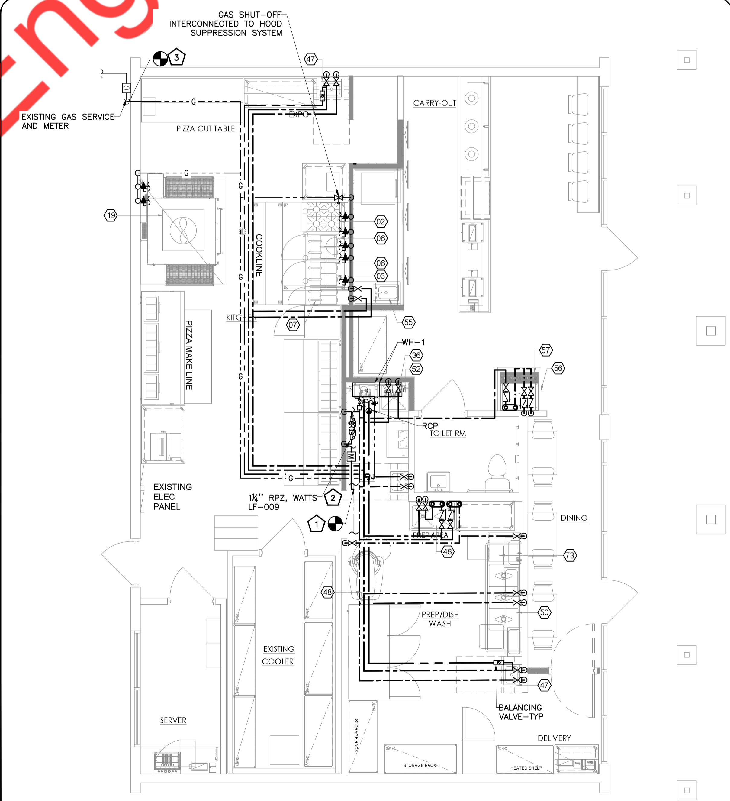
WATER/GAS PLAN SCALE 1/4" = 1'-0" 1
